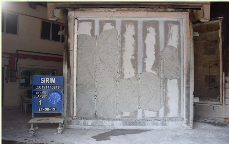
Photo 6 : The exposed face of the test specimen after the test
