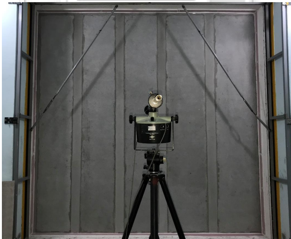
Figure 3 : “GEG ECO” lightweight wall panels system facing the receiving room
