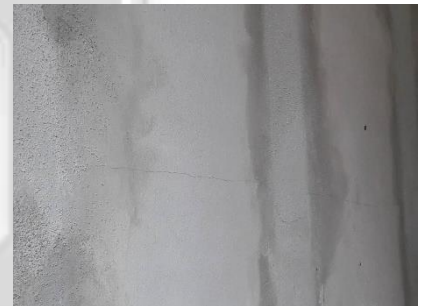
Figure 6 : Crack line observed at the back of partition wall at 7.5kN/m load applied.
