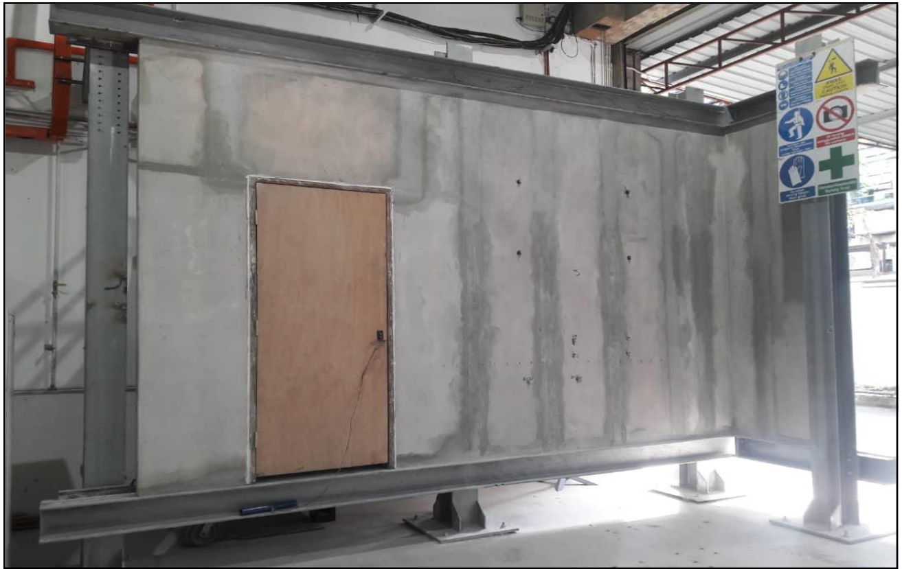
Figure 2: Test mock-up of GEG-ECO Light Weight Panel installed.
