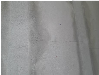
Figure 6 : Crack line observed at the back of partition wall at 7.5kN/m load applied.
