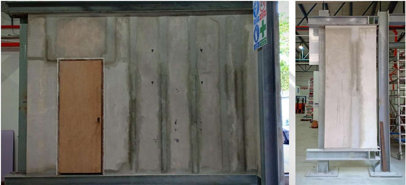
Figure 3: Test mock-up of GEG-ECO Light Weight Panel installed and right corner junction.
