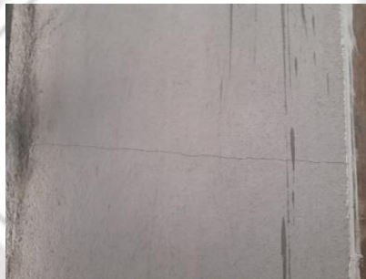
Figure 6 : Crack line observed at the back of partition wall at 7.5kN/m load applied.
