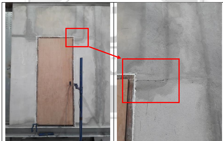
Figure 12: Hair line crack observed at plastering area on top right edge of the door during door slamming test
